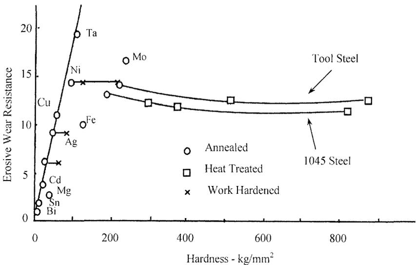
**Figure 20.9** Variation of erosive wear resistance with indentation hardness for various surface materials.
