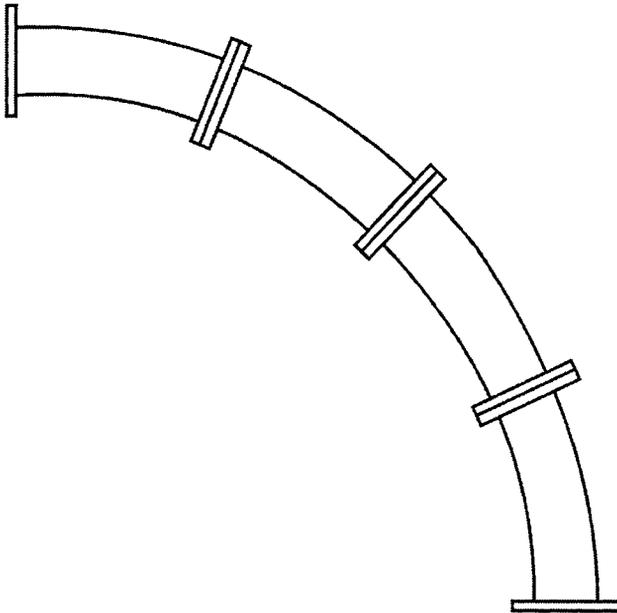
**Figure 20.15** Long radius bend with replaceable and interchangeable  $22\frac{1}{2}^\circ$  segments.
