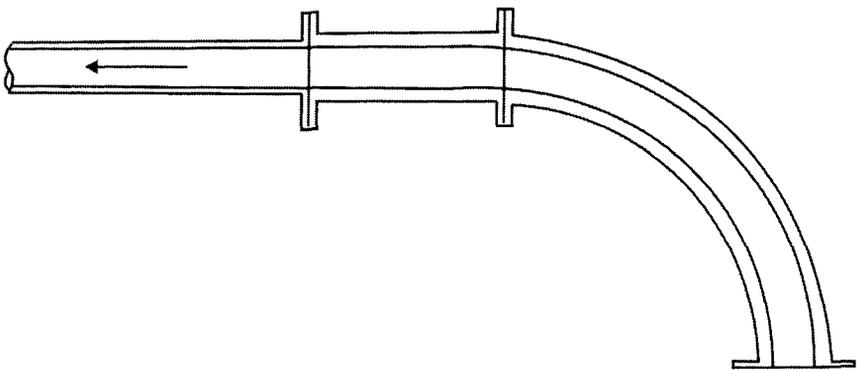
**Figure 20.27** Thick walled section of straight pipeline following reinforced bend.
