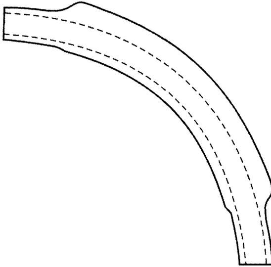
**Figure 20.26** Bend with reinforced walls.
