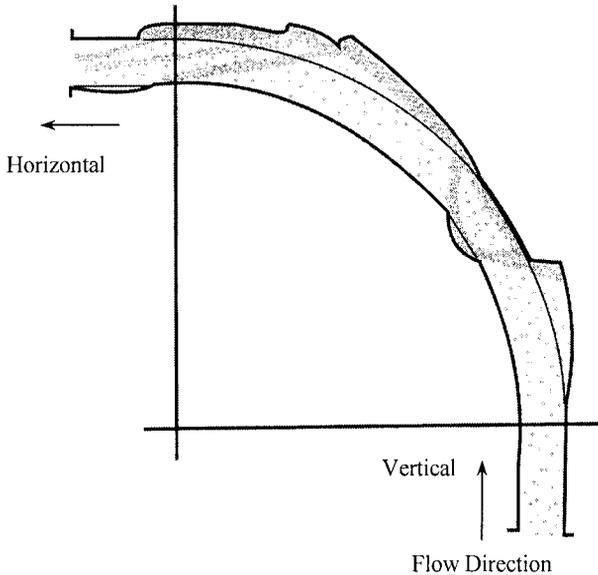
**Figure 20.25** Wear and flow pattern for an eroded bend.
