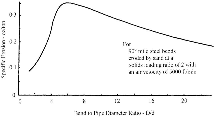
**Figure 20.13** The influence of bend geometry on the erosive wear of pipeline bends.
