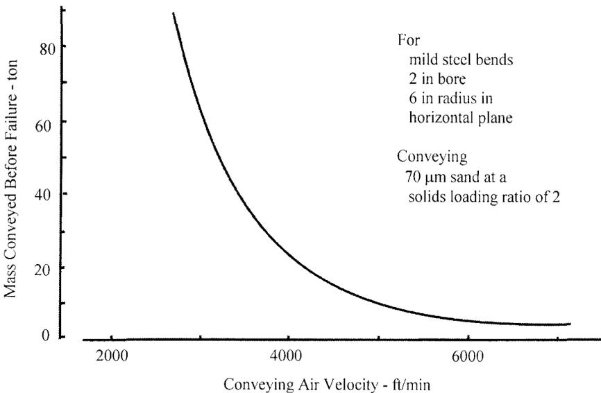
**Figure 20.4** The influence of velocity on the conveying capacity of the bends shown in figure 20.3.
