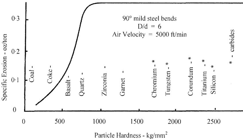
**Figure 20.7** The influence of particle hardness on the erosion of bends in a pneumatic conveying system pipeline.
