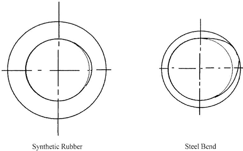
**Figure 20.20** Comparison of pipe section wear profiles for bends eroded by sand.
