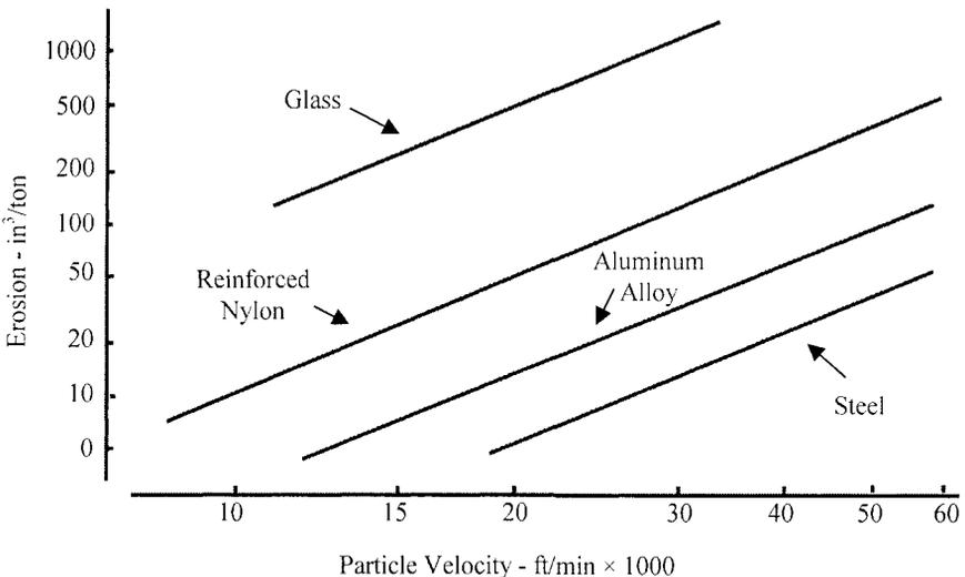
**Figure 20.2** Variation of erosion with velocity for various surface materials.
