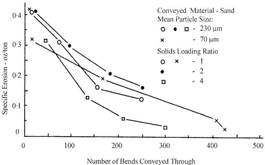
**Figure 20.12** The effect of particle degradation and wear on the erosion of bends in a pneumatic conveying system pipeline.
