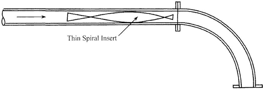
**Figure 20.22** Bend protection by use of sacrificial inserts in the preceding straight length of pipeline.
