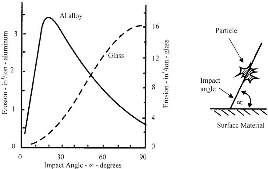
**Figure 20.1** Variation of erosive wear with impact angle for various surface materials.
