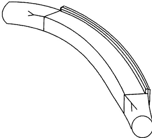
**Figure 20.24** Fabricated bend with square section and replaceable outer wall.
