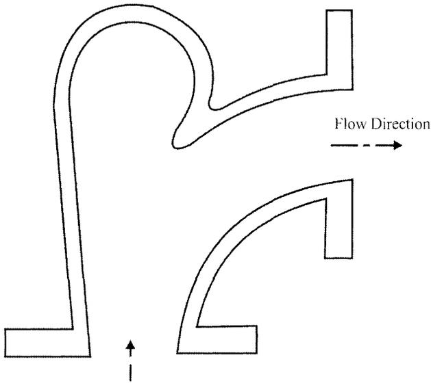
**Figure 20.18** Sketch of vortice pocket bend.
