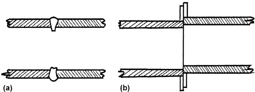
**Figure 20.28** (a) Welded and (b) flanged examples of erosion promoting sites at poorly jointed pipeline sections.
