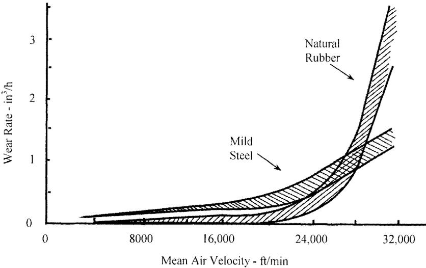
**Figure 20.10** The influence of air velocity on wear rate for mild steel and rubber surface materials.
