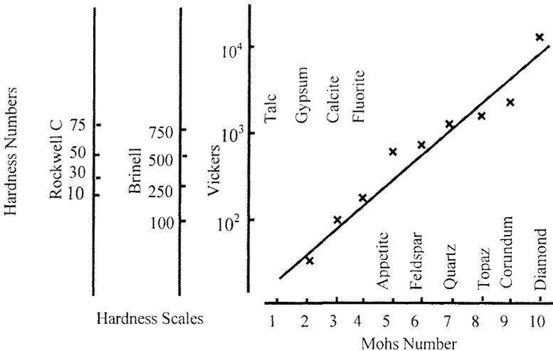
**Figure 20.8** Relationship between Mohs, Vickers, Brinell, and Rockwell hardness scales.
