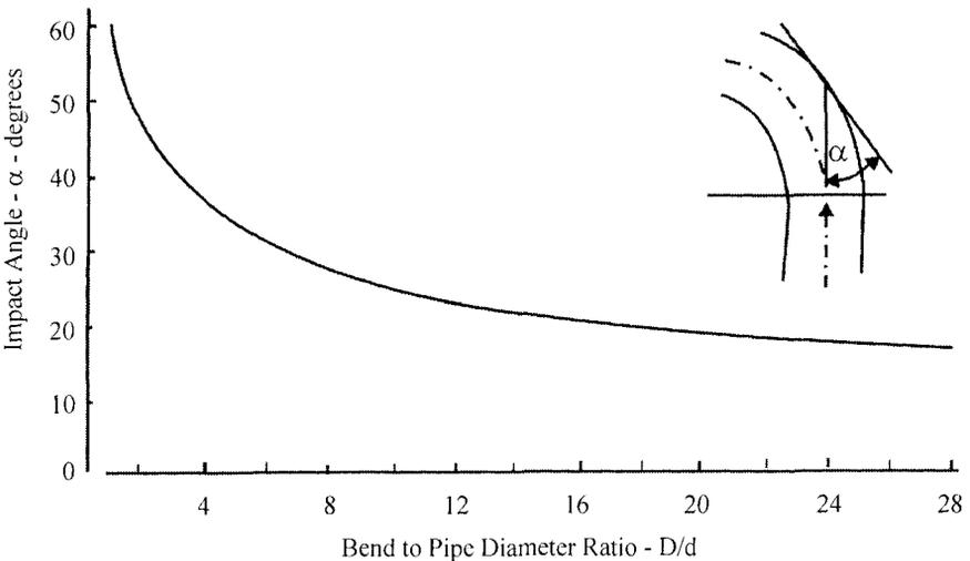
**Figure 20.14** Influence of bend geometry on particle impact angle.
