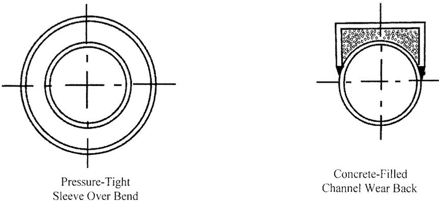
**Figure 20.21** Wear back methods of bend reinforcement.
