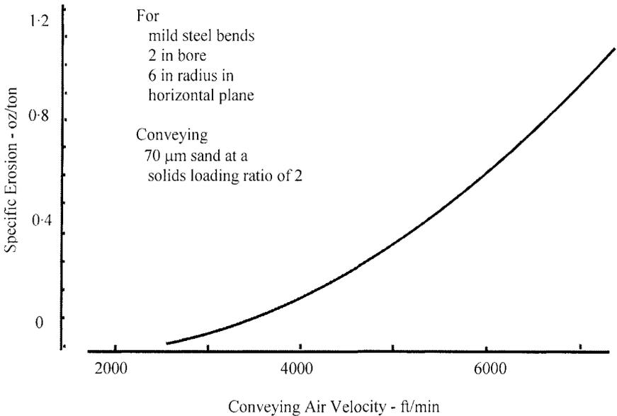
**Figure 20.3** The influence of velocity on the erosive wear of bends in a pneumatic conveying system pipeline.
