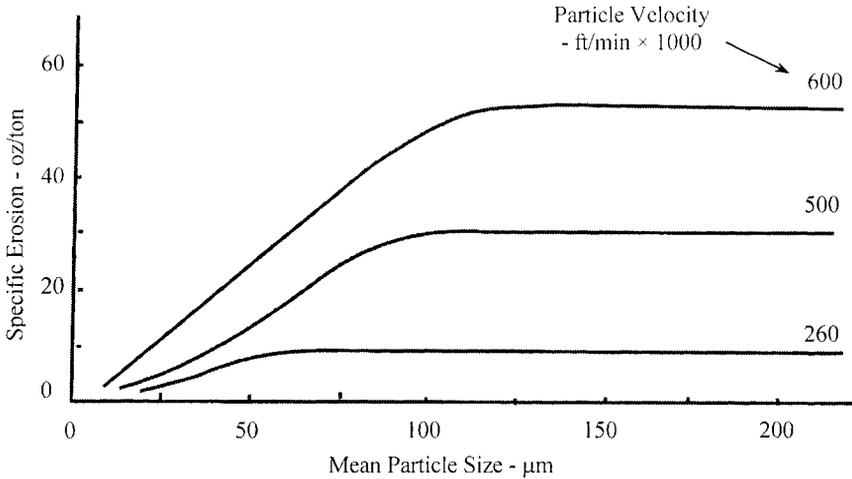
**Figure 20.5** The influence of particle size and velocity on erosion.
