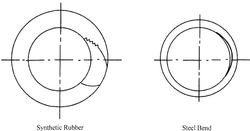
**Figure 20.19** Comparison of bend section wear profiles for bends eroded by coke.
