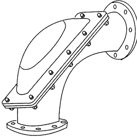
**Figure 20.23** Bend with reinforced and replaceable back.
