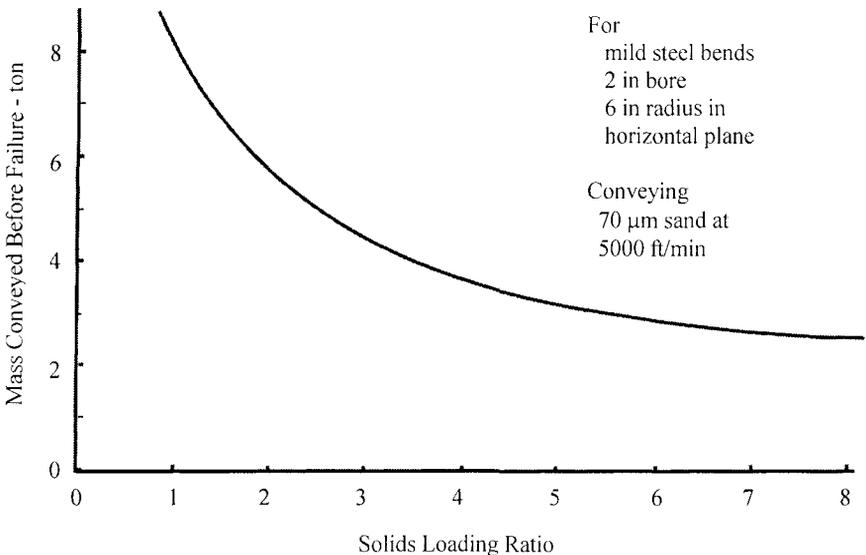
**Figure 20.11** The influence of solids loading ratio on the conveying capacity of bends in a pneumatic conveying system pipeline.
