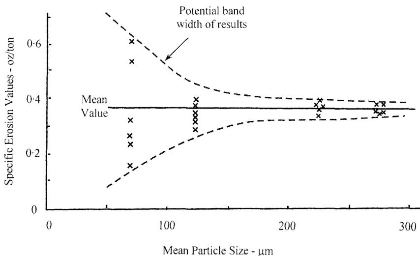
**Figure 20.6** The variation of individual specific erosion values with mean particle size for bends in a pneumatic conveying system pipeline.
