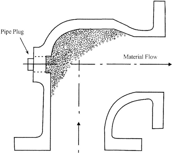
**Figure 20.17** Sketch of short radius bend with shallow depression.
